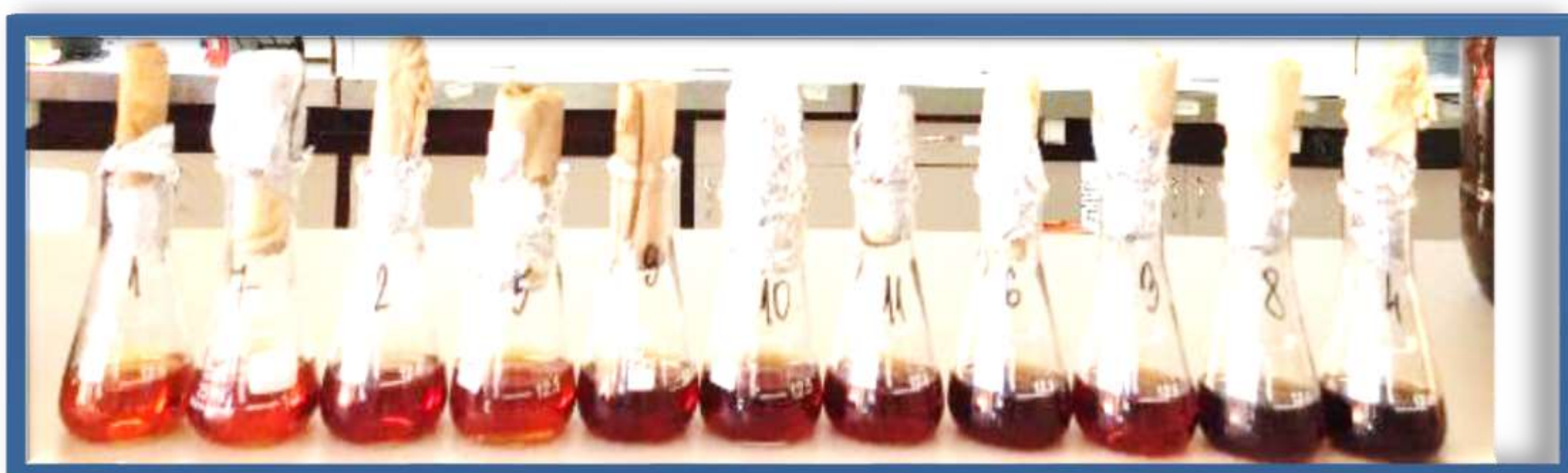
Figure 2. Qualitative analysis of polymerization of sample GA+EGCG+Commercial laccase with different time of incubation
